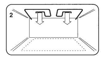
2. **Grilling (Top Oven)** - Has a full width, fully controllable grill. The grill also has an economy setting which enables you to use just the left section. NOTE: The oven door should be open when grilling. (See page "Operation when using the Top Oven for Grilling".)
